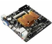
announced the J1900NH2 motherboard with the onboard Intel Dual-Core Celeron J1900 processor in a mini ITX form
